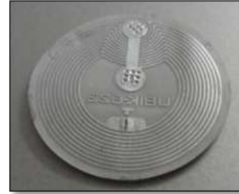
Fig. 5: The Sample NFC Tag - NTAG203
